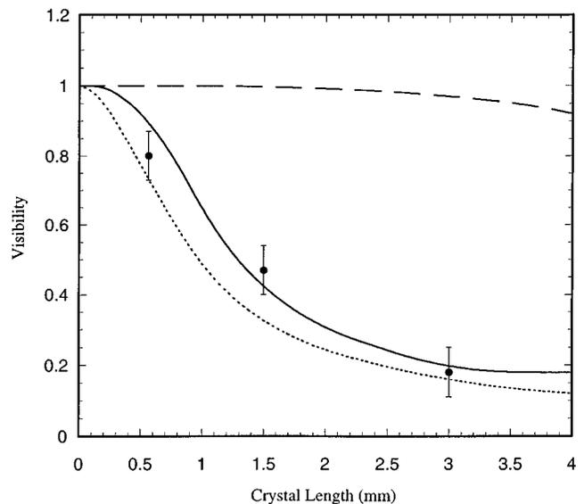
FIG. 3. Comparison of quantum interference visibility observed in the experiment with the results of theoretical prediction using 6-nm interference filters (solid line). Theoretical prediction with 0.6-nm interference filters (dashed line) and without any filters inserted (dotted line).
