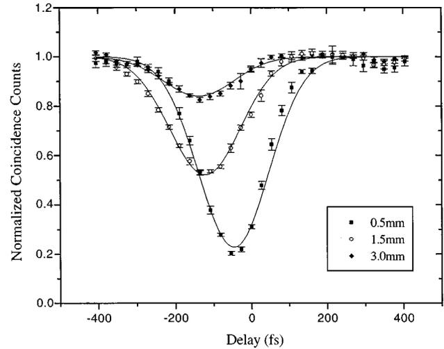
FIG. 2. Quantum interference measurement with three nonlinear crystals of different length 0.56, 1.5, and 3 mm.
