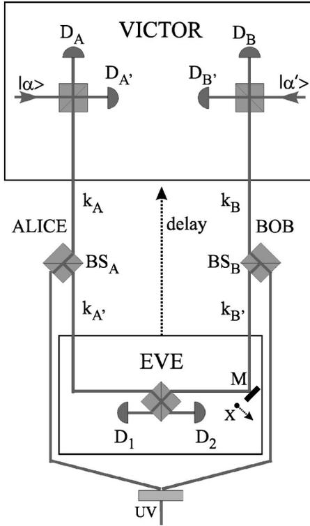
FIG. 1. Layout of an experimental demonstration of the delayed-choice entanglement-swapping process. In the actual experiment the two-homodyne apparatus was replaced by the two-detector set shown in Fig. 2, inset below.
