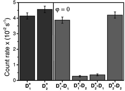
FIG. 3. Histograms showing the measured detection count rates by  $D_1^*$  and  $D_2^*$  and the accuracy affecting the experimental determination of the Bell states  $\Psi^\pm$  obtained by the delayed coincidence rates involving all detector pairs  $D_i^*-D_j$  ( $i, j=1,2$ ), for  $\varphi=0$ .
