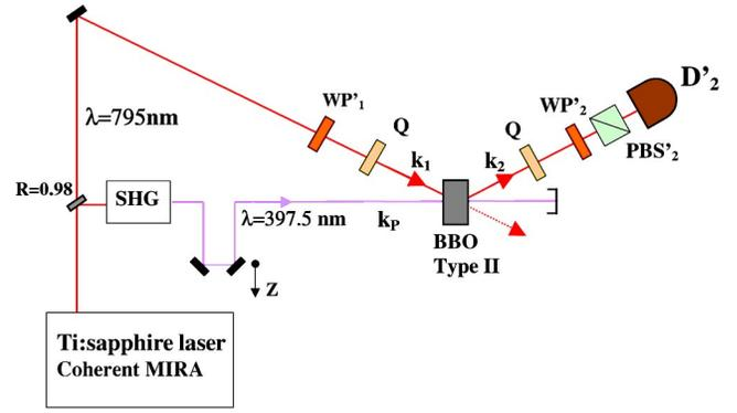
FIG. 3. (Color online) Injection apparatus of attenuated coherent optical pulses into a QIOPA to demonstrate the universality of the parametric amplification.
