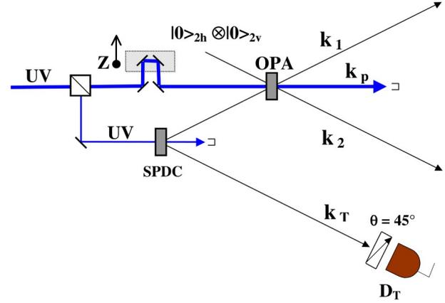
FIG. 2. (Color online) Schematic diagram of the *quantum-injected* optical parametric amplifier (QIOPA) in *entangled configuration*. The injection is provided by an external spontaneous parametric down conversion source (SPDC) of polarization ( $\pi$ ) entangled photon states.
