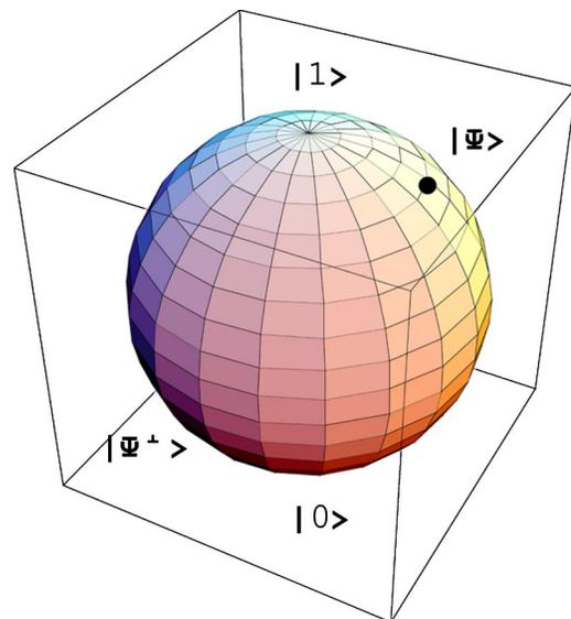
FIG. 1. (Color online) Bloch sphere, the state space of a quantum bit (*qubit*). *Pure states* are represented by points on the sphere while *statistical mixtures* are points inside the sphere. The universal-NOT gate operation corresponds to the inversion of the sphere, i.e., states  $|\Psi\rangle$  and  $|\Psi^\perp\rangle$  are antipodes.
