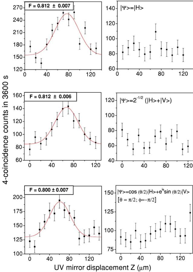
FIG. 6. (Color online) Demonstration of the UOQCM by single photon qubit self-injection and four-detector coincidences. The plots on the lhs and on the rhs of the figure mutually correspond. The rhs plots correspond to “noise”. The values of the fidelity of the process  $F$  evaluated by each test are expressed in the upper side of the lhs plots while the corresponding test qubits are expressed in rhs plots.
