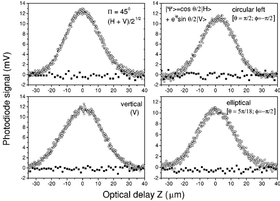
FIG. 4. Experimental verification of the universality of the OPA system by injection of  $\pi$  qubits represented by several significant points on the Bloch sphere. The injected state is encoded in a very attenuated coherent laser beam.
