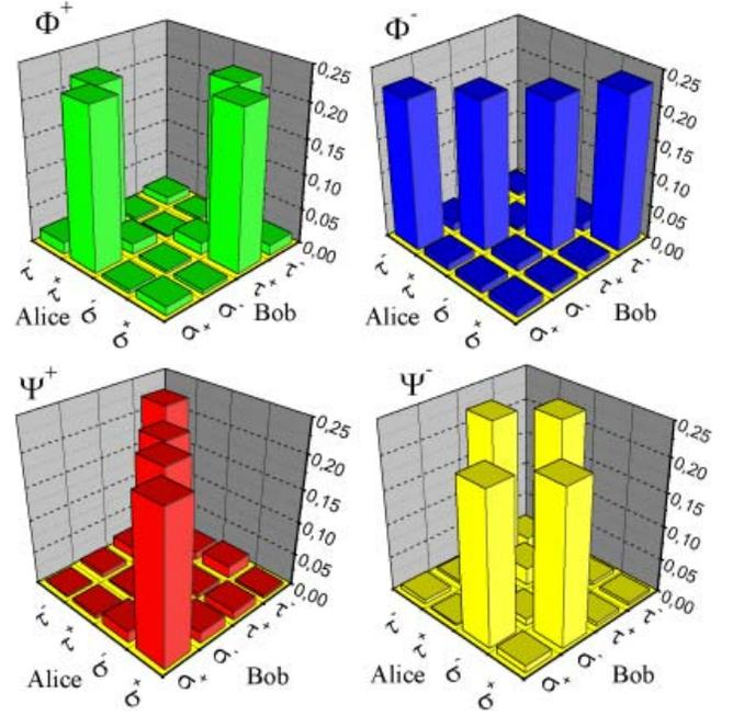
FIG. 2. (Color online) Experimental coincidence frequencies showing the complete Bell state analysis of the polarization states  $|\Phi^+\rangle$ ,  $|\Phi^-\rangle$ ,  $|\Psi^+\rangle$ ,  $|\Psi^-\rangle$ . Relative errors are typically 2% for the maxima and 5% for the other terms.
