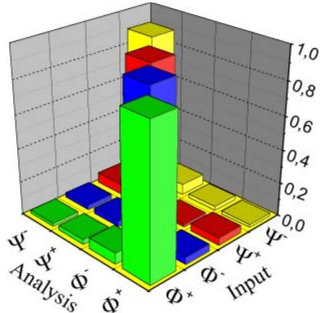
FIG. 3. (Color online) Overall experimental fidelities obtained by the Bell state analyzer for each input Bell state. Relative errors are typically 2% for the maxima and 5% for the other terms.
