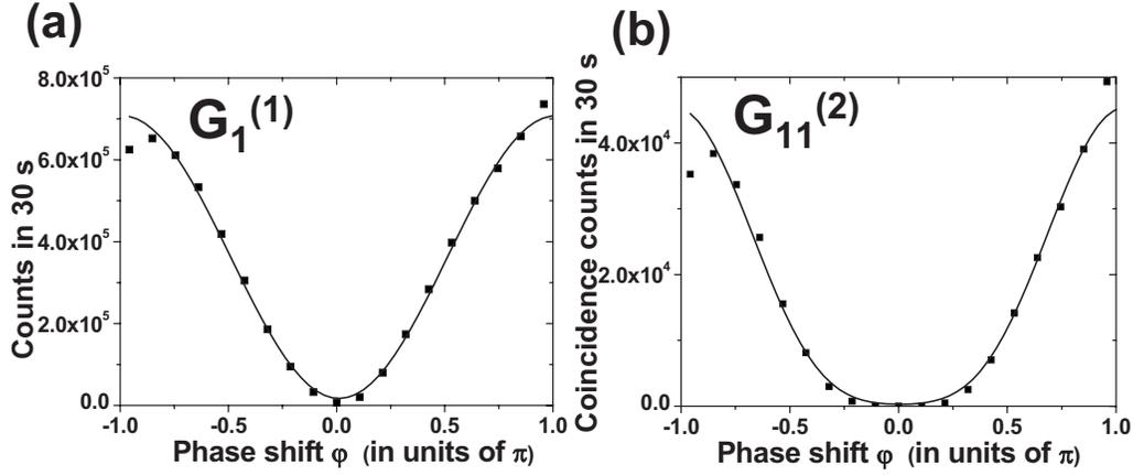
FIG. 3. Coherent state as input field. (a)  $G_1^{(1)}$ : Count rates  $D_1^A$  versus the phase  $\varphi$ . (b)  $G_{11}^{(2)}$ : Coincidence counts  $[D_1^A, D_1^B]$  versus the phase  $\varphi$ .
