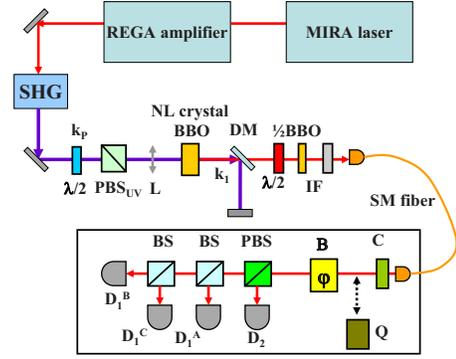
FIG. 2. (Color online) Experimental layout. The radiation generated in the NL crystal is spectrally filtered by an interferential filter (IF) with bandwidth equal to 3 nm and spatially selected adopting a single mode (SM) fiber.
