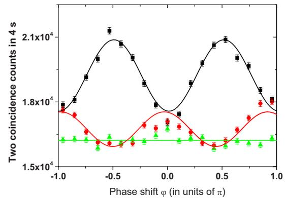
FIG. 7. (Color online) Effects of coherence on fringe visibility. Square data: Two-photon coincidences counts versus the phase  $\varphi$  without introducing decoherence. Circle data: Decoherence introduced between the polarization components  $\{\vec{\pi}_H, \vec{\pi}_V\}$ . Triangle data: Decoherence introduced between  $\{\vec{\pi}_+, \vec{\pi}_-\}$ .
