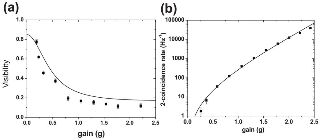
FIG. 5. (a) Visibility versus nonlinear gain. The continuous line corresponds to the function  $V_{\max} \times V_1^{(2)}(g)$ . (b) Excitation rate versus nonlinear gain. The continuous line corresponds to the function  $\bar{R}^{(2)}(\alpha g)$ , where the parameter  $\alpha$  has been optimized by fitting the data and reads as 0.85.
