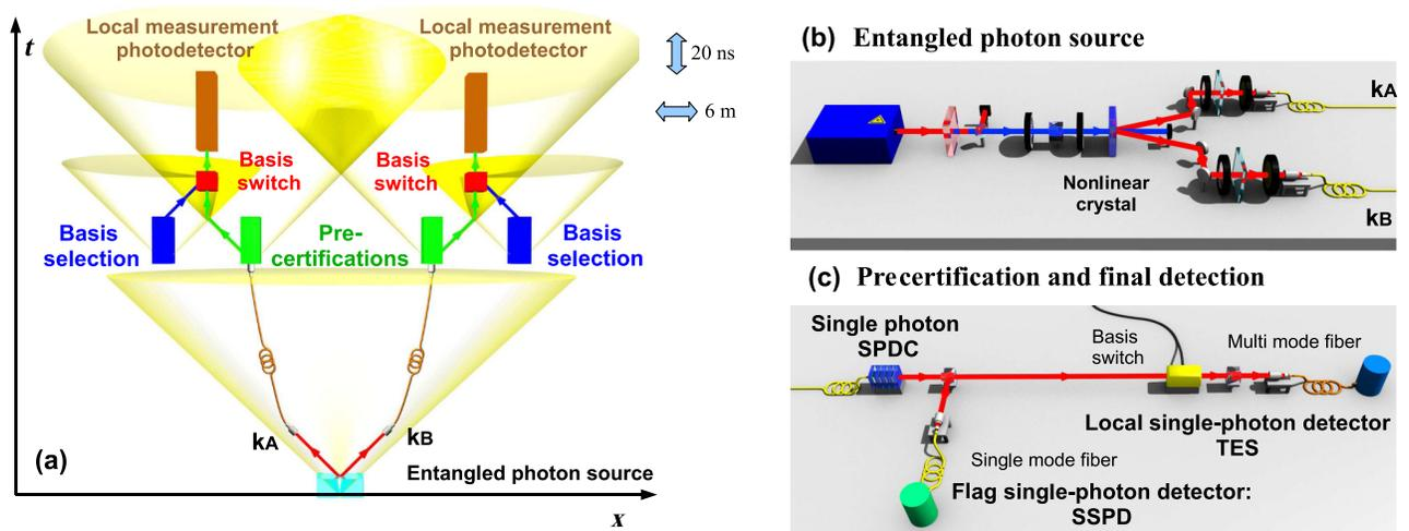
FIG. 1. (a) Space-time diagram of a Bell test based on local precertification of the photon’s presence. Green box: Precertification stage. Blue box: Basis selection. Red box: Measurement process. Orange box: Final measurement stage. (b) Source of polarization-entangled states. (c) Precertification and detection apparatus.
